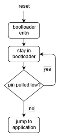
Another method supported by booty is to stay in the bootloader for a time after reset or after the most recent valid message has been received. This method has the advantage of requiring no additional hardware, but the disadvantage of slow application startup time.
